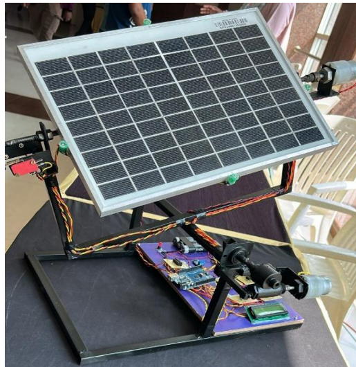
Figure 3. Fabricated prototype of the proposed dual-axis solar tracking system
