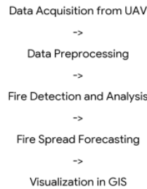
Figure 1. Architecture of the GIS for forest fire monitoring
